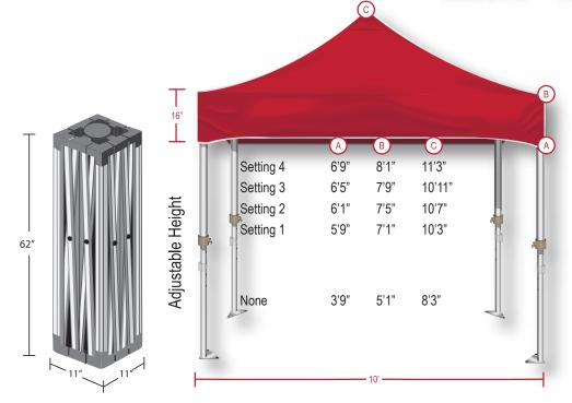
The XTF frame is another first for KD Kanopy, bringing a heavy duty canopy to the market but keeping the price budget friendly. Using new nylon composite fittings means no binding and an easy glide motion. The pull pin release makes the canopy even easier to setup and tear down. The industrial coil spring on the outside of the center pole guarantees supreme tension in your canopy which helps shed rain fall and gives a more professional, clean look to your canopy. Frame weighs 56 lbs.
